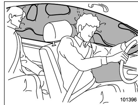
The driver's and front passenger's SRS side airbags and SRS curtain airbags deploy independently of each other because each has its own impact sensor. Therefore, they may not both deploy in the same accident. Also, the SRS side airbag deploys independently of the driver's and front passenger's SRS frontal airbags in the steering wheel and instrument panel.
