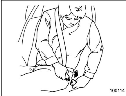
5. Insert the center seatbelt tongue plate into the center seatbelt buckle until it
