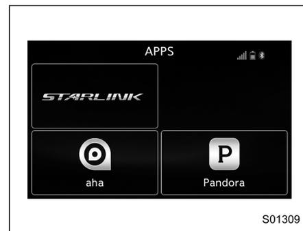
3. Touch the "STARLINK" key on the APPS screen. The disclaimer screen or the error screen is displayed.
